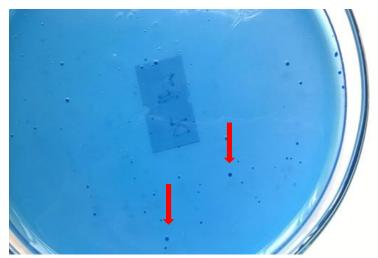
**Figure 1.** Colonies of the isolated strains on CMC agar, supplemented with 25 mg L<sup>-1</sup> methylene blue Arrows indicate the colonies that were selected as potential lignin-degrading bacteria.
