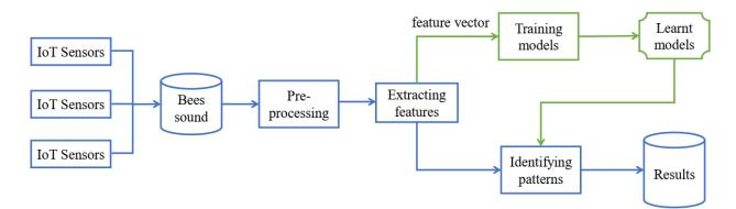
Figure 1. The architecture of audio-based beehive monitoring system
