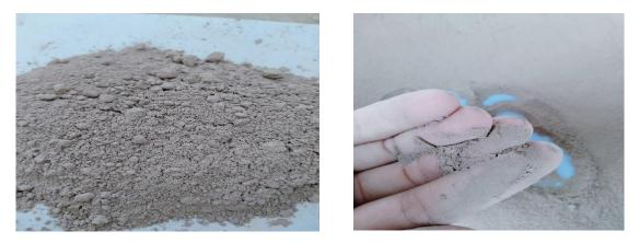
Figure 1. Fly ash collected from an ESP system at the Mong Duong 2 thermal power plant
