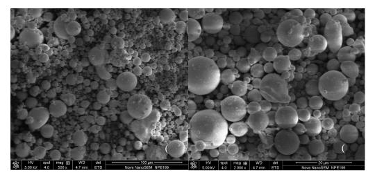
Figure 3. Scanning electron micrographs of the fly ash at (a) 500x and (b) 2000x magnification
